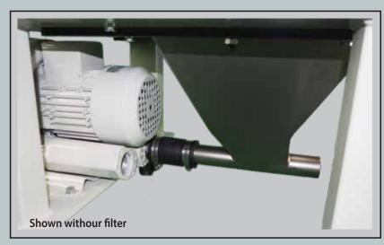
Our custom system includes a blower; air intake filter and cover; base; collection bin; and custom electrical controls. Evacuation hose is not included.
