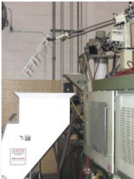
Sprue Picker Robot with SRS Bi-Cutter Screenless Granulator
