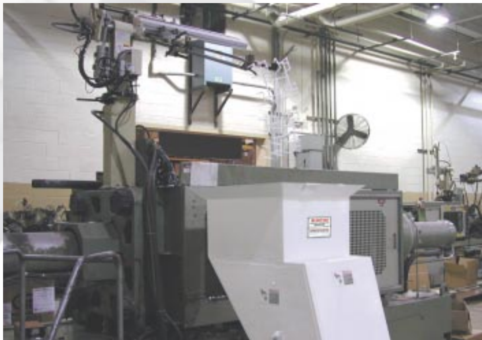
Sprue Picker Robot with SRS Bi-Cutter Screenless Granulator at Rodon Group Plant
